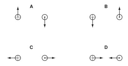
**32** A simple model of a d.c. motor is made. By mistake, the split-ring commutator is left out. The coil can turn, but is always connected to the battery in the same way.
